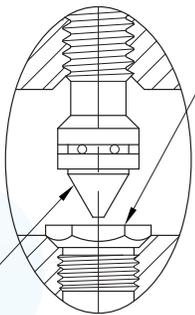
ÁGUA FLOTANTE REEMPLAZABLE ACERO INOXIDABLE
